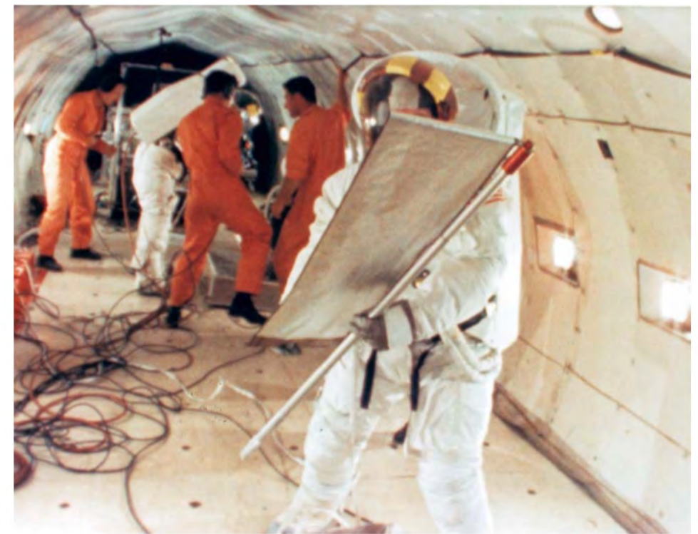
Figure 6. Astronaut Don Lind testing the deployment of the SWC instrument at 1/6 g in a B-707 airplane of NASA.
