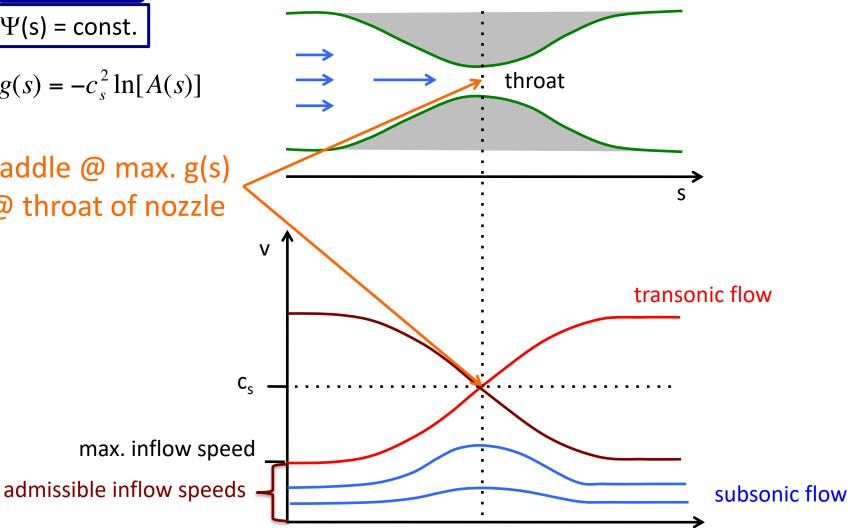
$g(s) = -c_s^2 \ln[A(s)] + \Psi(s)$ tube: horizontal nozzle  $\Psi(s) = const.$  $\mathbf{w}_{\text{exit}}$  $g(s) = -c_s^2 \ln[A(s)]$  $W_{o}$ Speeds up Slows down approaching in flaring exit constriction Inflow = mass loss rate set by back-pressure  $\mathbf{W}_{\text{exit}}$ subsonic flow tube:
