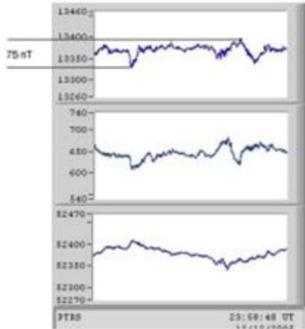
Petersburg, AK magnetometer data with a 75 nT change in the X-direction (Magnetic North)
