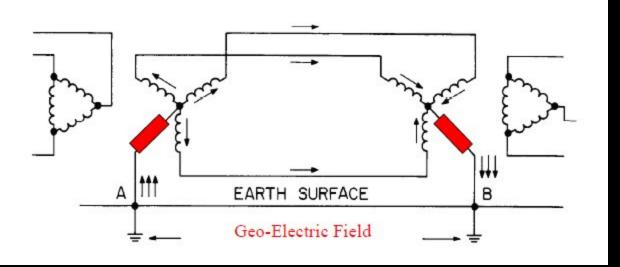
Adding resistors to ground lines
