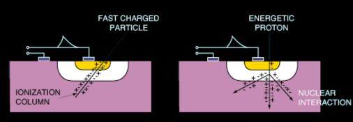
Excess charge causes gate state change
