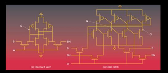
A six-transistor latch, commonly used as the storage element in a static memory circuit, is shown alongside a design-hardened 12-transistor variant. (Courtesy Aerospace Corp)
