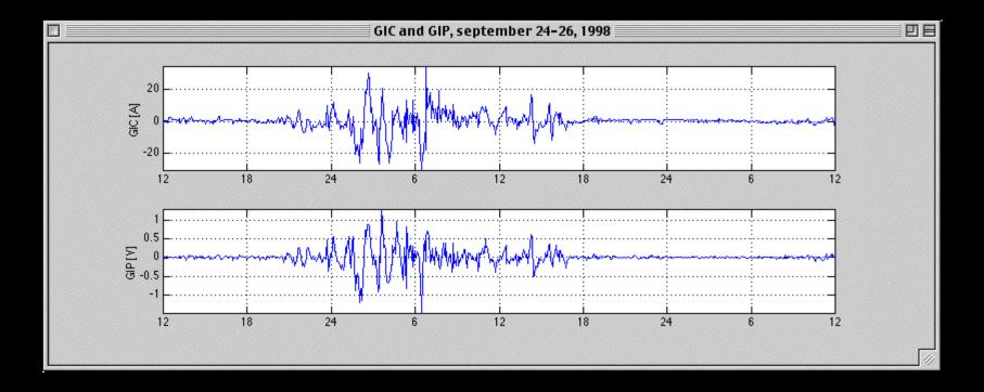
Top = GIC in 400 kV transformer ground – southern Sweden Bottom – GIC in natural gas pipeline – southern Sweden
