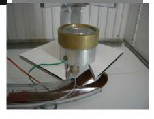
Inner ring melts clean ice; outer ring collects waste water. Capillary slits minimize upward wicking
