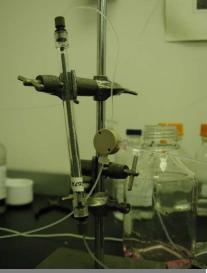
Meltwater with eluents pass through cadium reaction column before nitrate analysis.
