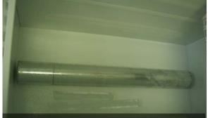
Quartered cores are repackaged, brought to ice core analysis lab at CSP on BU's main campus, and stored in chest freezer
