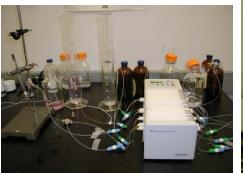
Multichannel peristaltic pump provides throughput. Carrier and reagent is mixed with meltwater for nitrate analysis. Pure portion of melt is diverted to conductivity meter.
