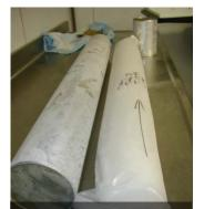
Cores bagged in field; note "this-end-up" arrow
