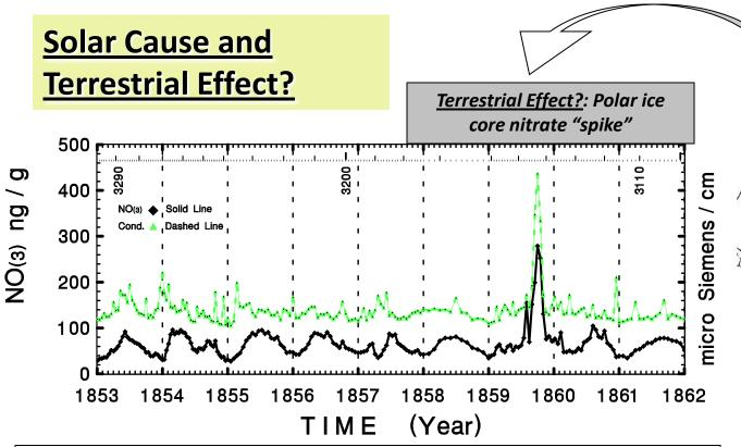
Example of high-resolution nitrate concentrations (black curve in ng  $g^{-1}$ ) and electrical conductivity (green curve in mSiemens cm<sup>-1</sup>) from the Greenland ice core. The large impulsive event at 1859.75 is the largest such event in the period 1561-1991 and occurs in close correlation to the extremely rare 1 September 1859 "white light" flare observed by Carrington (1860). (Taken from Shea and Smart, 2003)<sup>(18)</sup>
