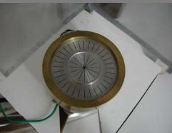
Melt water is pumped out of freezer for analysis; depth of core is recorded during each melt
