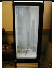
Firn melter temperature controlled by heaters w/ active feedback
