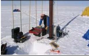
Two proximate 30-meter-deep cores were finished on June 9th at Summit, Greenland by Jay Kyne, a driller with Ice Core Drilling Services, using a 4" "SideWinder" drill.
