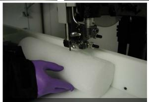
At 30-meters core is "firn", compacted snow
