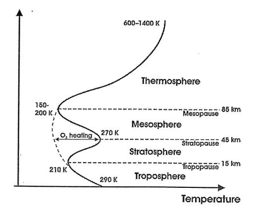
Average vertical temperature profile through Earth's atmosphere. The general shape of the temperature profile is reasonably consistent, to the point where it can be used to define the four main neutral-atmosphere "layers", from the troposphere to the thermosphere.
