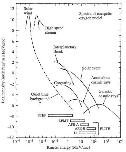
An illustration of the energy spectrum of cosmic rays in the heliosphere based on spacecraft observations.
