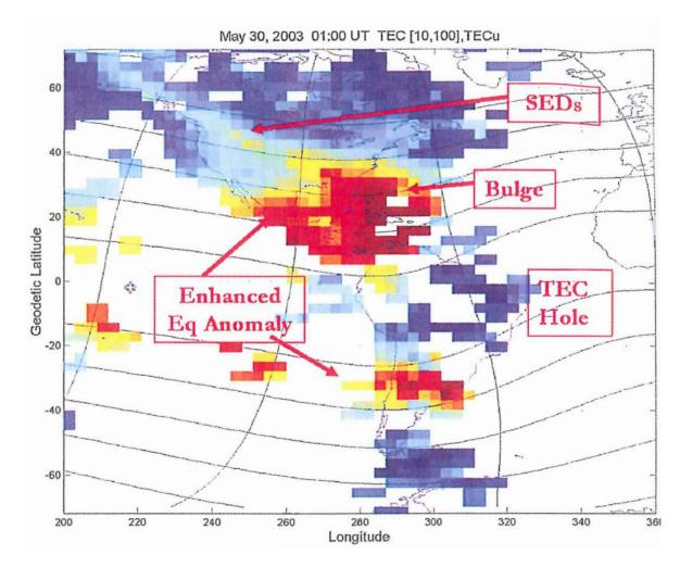
Illustration of the large enhancement "bulge" in TEC at mid-latitudes during a geomagnetic storm, and showing the plume of plasma (storm-enhanced density, or SED) connecting the bulge to the high latitudes. (Courtesy of J. Foster.) *Book 2, pp. 339.*
