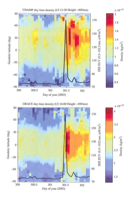
Thermospheric density enhancements measured by accelerometers on the CHAMP satellite (altitude ~400 km) and GRACE satellite (altitude ~490 km) during the October 28, 2003 flare. (Sutton et al., 2006.)
