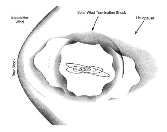
The heliosphere is the sphere of influence carved out by the Sun in the surrounding interstellar medium. The solar wind flows out incessantly in all directions, past the orbiting planets, and is finally halted at the termination shock (the innermost nested surface). The shocked solar wind material diffuses outward into the surrounding material forming the heliopause (the prolate spheroid that encloses the spherical termination shock.
