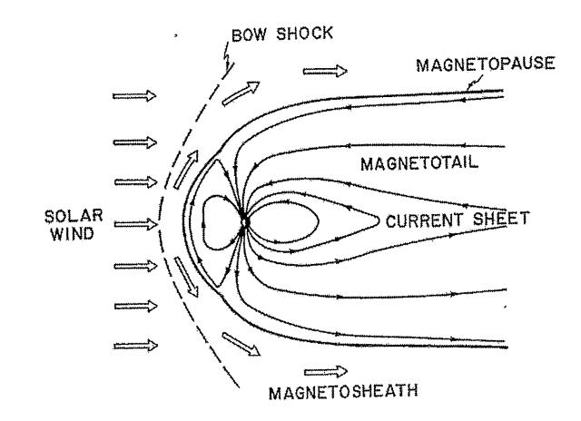
Schematic view of a magnetically closed magnetosphere, cut in the noonmidnight meridian plane. Open arrows, solar wind bulk flow; solid lines within magnetosphere, magnetic field lines (directions appropriate for Earth).
