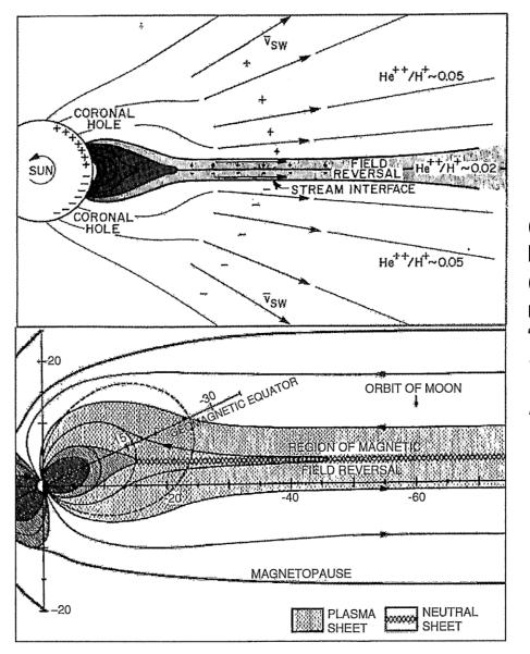
(Upper panel) The heliospheric current sheet, labeled "field reversal", and its plasma sheet (Gosling et al., 1981) and (lower panel) the magnetospheric current sheet, here the "neutral sheet", and its plasma sheet (Ness 1969.)
