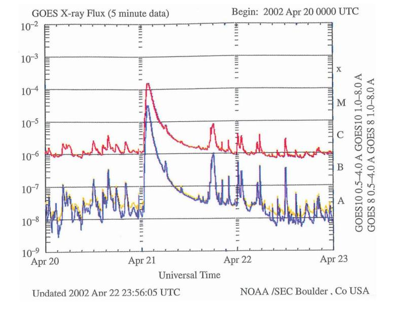
Example of GOES XRS measurements during a large (X1.5) solar flare.
