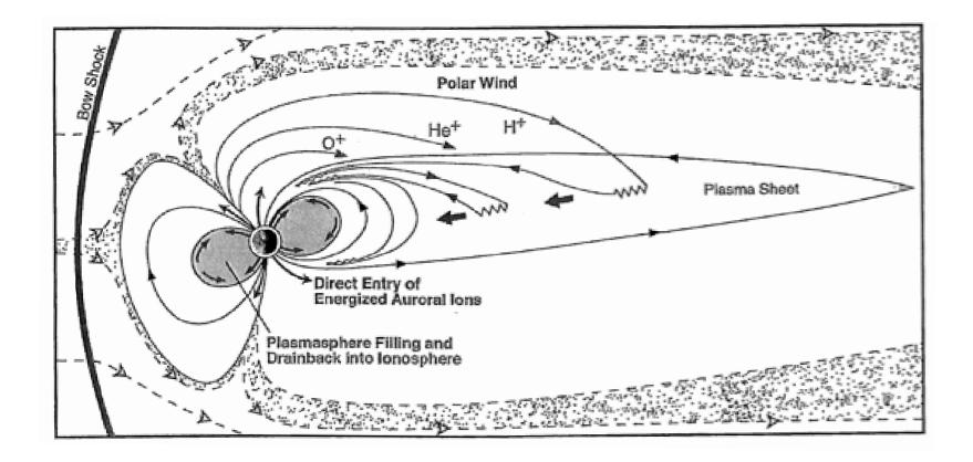
Sources of plasma for the Earth's magnetosphere (after Chappell, 1988). The shaded and dotted area illustrates the boundary layer through which solar wind plasma enters the magnetosphere.
