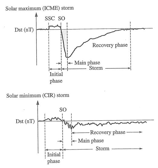
Schematic time history of geomagnetic field variation for two characteristic magnetic storms. Time range; several days. Vertical variation range: ~100–200 nT. SSC: storm sudden commencement. SO: storm onset. The top panel shows the storm development in response to a characteristic interplanetary coronal mass ejection (ICME), and the bottom panel that for the passage of a corotating intersection region (CIR). (Figure adapted from Tsurutani et al., 2006.) *Book 2, pp. 264.*
