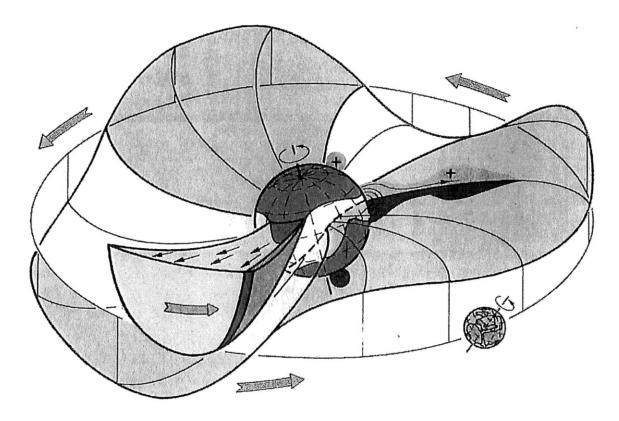
The heliospheric current sheet forms a warped, undulating structure extending from the top ridge of the helmet streamer belt (cf. Figs. 1.3 (top panel) and 8.1) that sweeps by the Earth as the Sun rotates once per 27 days (the synodic period).
