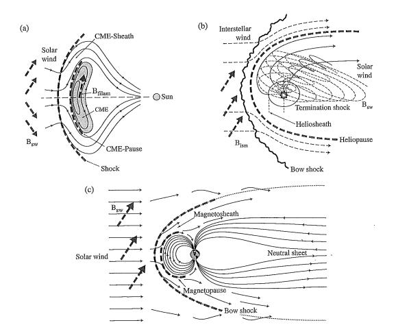
Schematic comparison of shocks around CMEs, the heliosphere, and the magnetosphere. The figure shows some of the types of shocks and sheaths that exist in the heliosphere and their universal basic structures; (a) a CME, (b) the outer heliosphere, and (c) Earth's magnetosphere.
