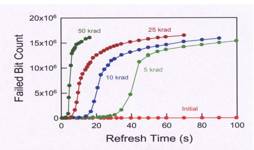
Figure 66: Number of failed bits versus refresh time for 16 Mb DRAMs irradiated with Co-60 gamma rays at total doses from 0 to 50 krad(Si). (After Ref. [219])
