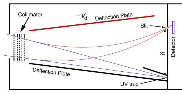
The main advantage of a SADA is that particles up to several MeV/charge can be deflected since K can be large and large deflection voltages can be supported
